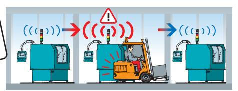
The siren element adjusts its sound output through continual measurement of the ambient noise level. The emitted tone is c. 5 dB louder than the background sound level. The warning signal can always be heard without being irritatingly loud for people in the sounder's vicinity.
