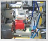
Gentle removal of the injection moulded parts using a gripper arm.
