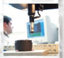
Checking the injection moulded parts with the assistance of a 3D coordinate measuring machine.
