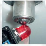
Shock resistance test: A weight falls from a precisely defined height onto the beacon
